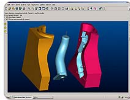
Left: ZCast mold and aluminum pipe created using the ZCast technology. Above: Screen shot of ZCast mold and core set created in 3D CAD.
